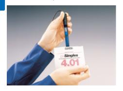
ICN Oakton® pH Singles are calibration solution pouches containing 20 ml of pH calibration solution or deionized water for rinsing. All solutions are certified traceable to NIST standards for maximum accuracy. Pouches are airtight, guaranteeing freshness for each use. Each pouch is labeled with the name and CAS number for all ingredients to conform with "Right-to-Know" requirements.
