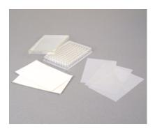
Acetate plate sealers are NON gas permeable and mylar plates are gas permeable. All sealers are supplied non-sterile, and they are not autoclavable. The dimensions are approximately 13.3 x 8.3 cm.
